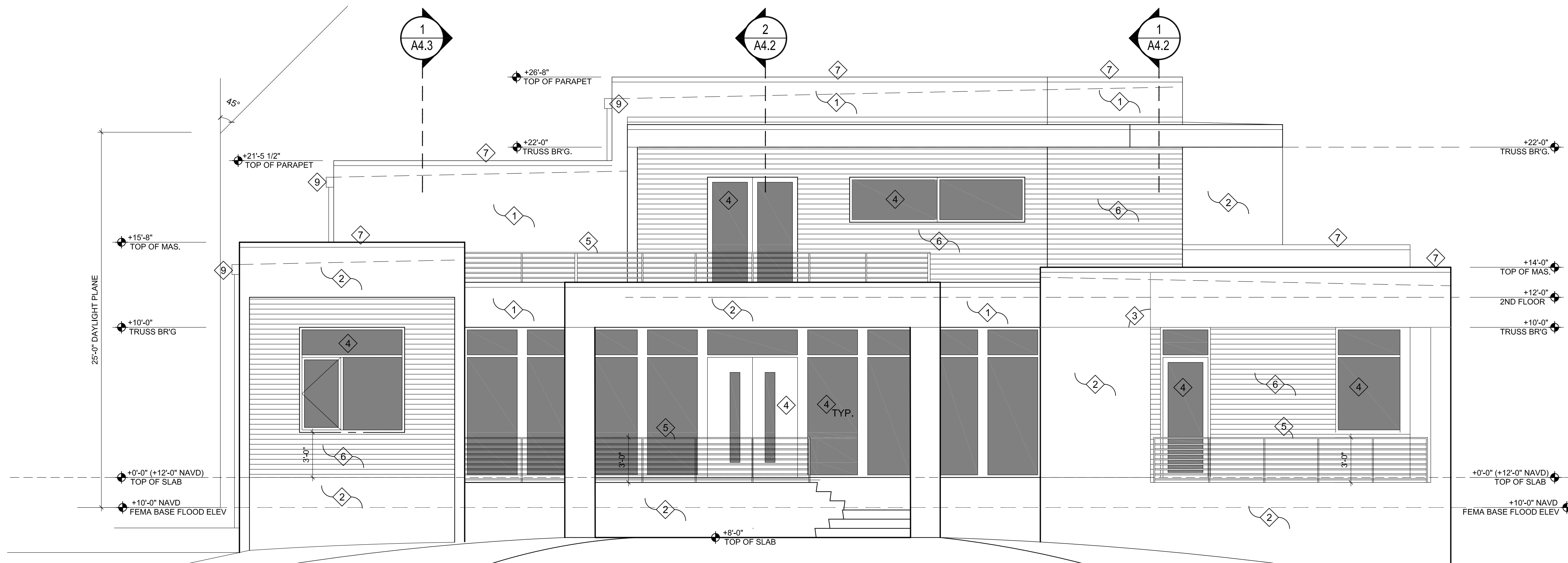
NORTH ELEVATION SCALE: 1/4" = 1'-0"
